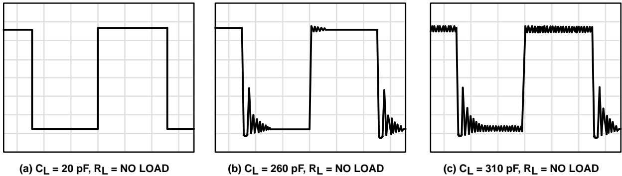
Figure 112. Effect of Capacitive Loads in Low-Bias Mode
