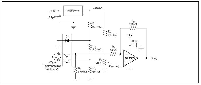
FIGURE 3. Temperature Measurement Circuit.
