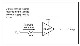
FIGURE 1. Input Current Protection.
