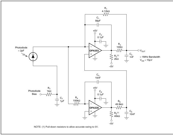
FIGURE 8. High Dynamic Range Transimpedance Amplifier.
