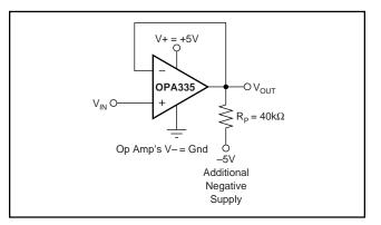
FIGURE 2. Op Amp with Pull-Down Resistor to Achieve  $V_{OUT}$  = Ground.
