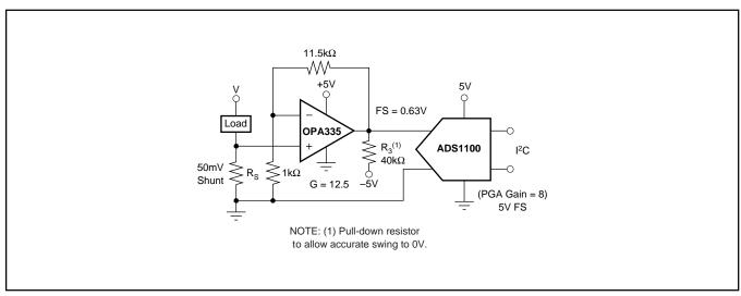
FIGURE 7. Low-Side Current Measurement.
