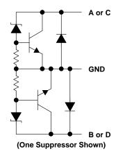
NOTE A: All four GND terminals should be connected to ground.
