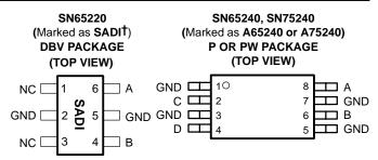
NC – No internal connection TWhen read horizontally, Pin 1 is the bottom left pin.
