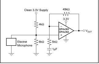
FIGURE 10. Microphone Preamplifier.
