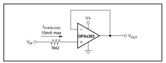
FIGURE 4. Input Current Protection.
