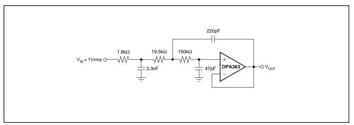
FIGURE 12. The OPA363 or OPA364 Configured as a 3-Pole, 20kHz, Sallen-Key Filter.
