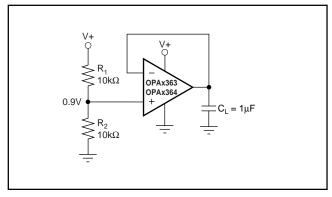
FIGURE 6. The OPA363 and OPA364 Provide a Stable Reference Voltage.
