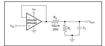
FIGURE 3. Improving Capacitive Load Drive.
