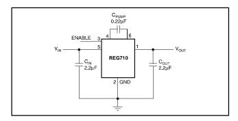
**Figure 3. Typical Operating Circuit**
