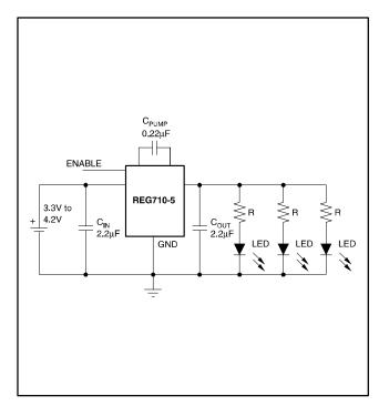
Figure 7. REG710 Circuit for Driving LEDs
