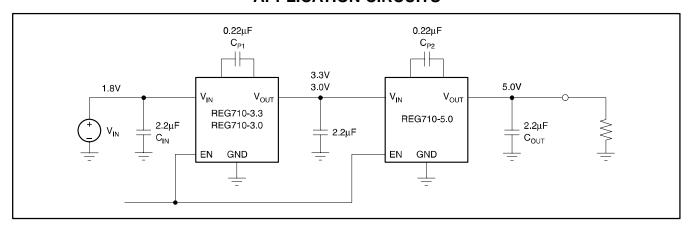
Figure 5. REG710 Circuit for Step-Up Operation from 1.8V to 5.0V with 10mA Output Current
