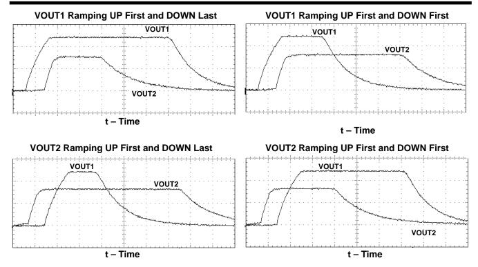
Figure 1. Example Voltage Ramp-up/Ramp-down Sequences
