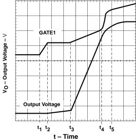
Figure 5. TPS2306 Typical IMAX1 Turn-on Sequence
