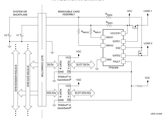
Figure 8. Using the TPS2306 with Bus Switches
