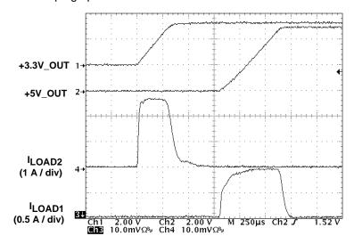
Figure 3. TPS2306 Output Ramp Operation in Figure 2 Circuit.
