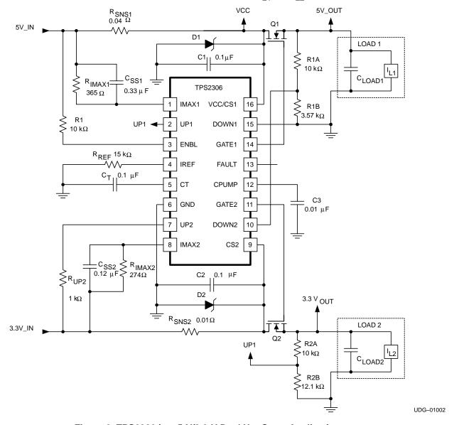
Figure 2. TPS2306 in a 5-V/3.3-V Dual Hot Swap Application
