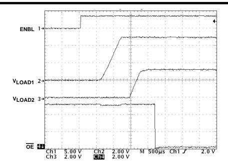
Figure 9. TPS2306 FAULT Operation During Ramp-Up
