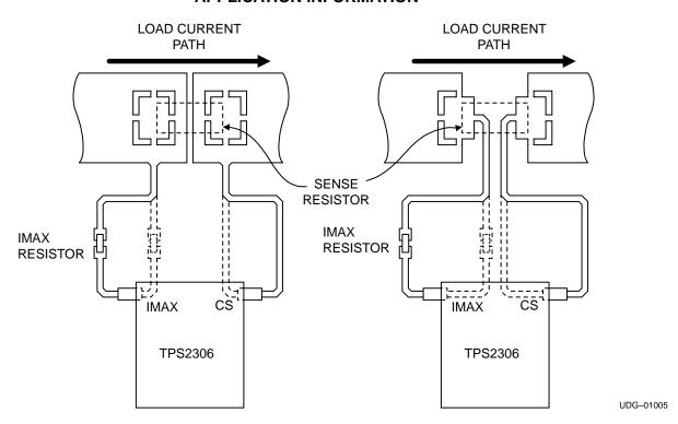
Figure 4. Connecting to the Sense Resistors—SMD Chip
