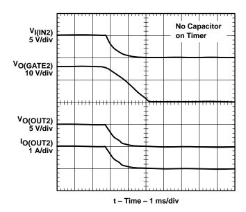
Figure 14. Channel 2 - Hot Removal
