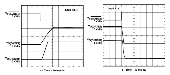
Figure 1. Turnon Voltage Transition of Channel 1
