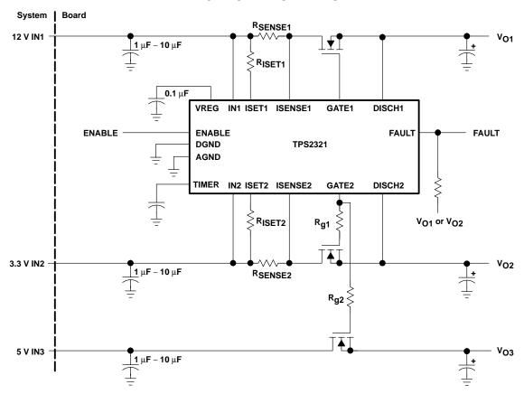
Figure 27. Three-Channel Application
