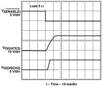
Figure 3. Turnon Voltage Transition of Channel 2
