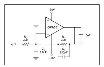
FIGURE 7. Driving Large Capacitive Loads.
