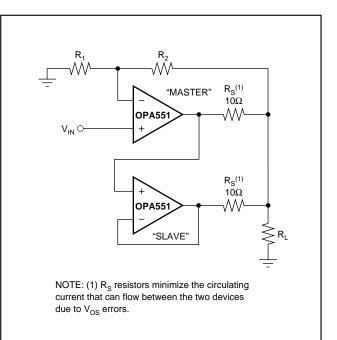
FIGURE 9. Parallel Amplifers Increase Output Current Capability.
