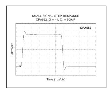
FIGURE 12. Small-Signal Step Response for Figure 11.
