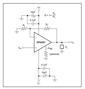
FIGURE 1. Basic Circuit Connections.
