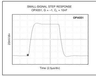
FIGURE 8. Small-Signal Step Response for Figure 7.
