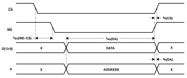
**Figure 3. Write Timing**
