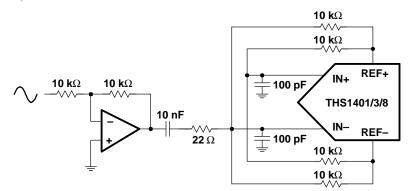
Figure 22. Single-Ended With Level Shift
