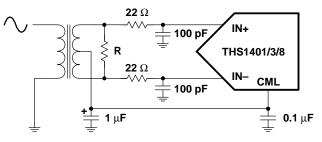
Figure 20. Transformer Coupled
