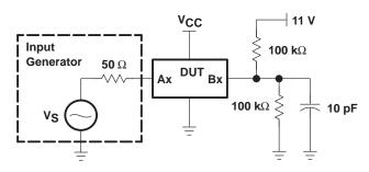
Figure 1. Device Test Setup
