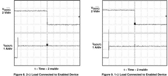
Figure 8. 2-Ω Load Connected to Enabled Device
