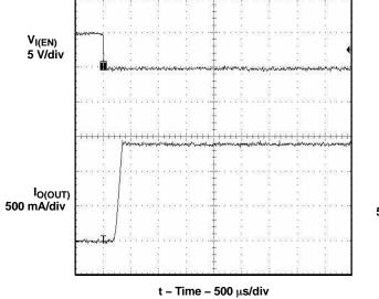
Figure 6. Short-Circuit Current, Device Enabled Into Short
