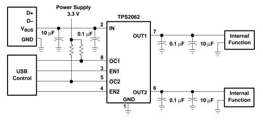
Figure 28. High-Power Bus-Powered Function
