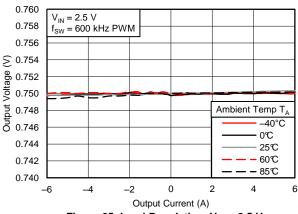
Figure 25. Load Regulation, V<sub>IN</sub> = 2.5 V
