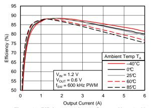
Figure 16. Efficiency vs. Output Current,  $V_{IN} = 1.2 \text{ V}$
