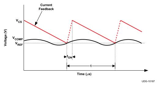
Figure 3. D-CAP+™ Mode Basic Waveforms
