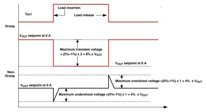
Figure 8. DROOP vs Non-DROOP in Transient Voltage Window
