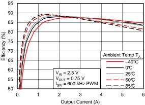
Figure 19. Efficiency vs. Output Current, V<sub>IN</sub> = 2.5 V
