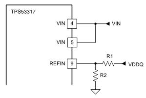
Figure 13. Tracking Configuration 1
