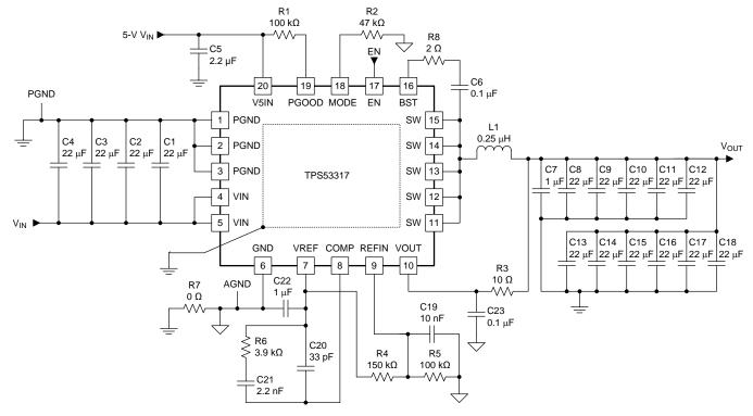
Figure 40. Design Example 3 Schematic: Non-Tracking POL Application
