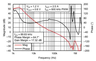
Figure 35. Bode Plot, No Load
