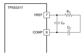
Figure 31. Compensation Network Circuit
