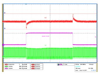
Figure 5. Load Regulation for 1.5-V Input, 0.75-V Output (Non-Droop Configuration)
