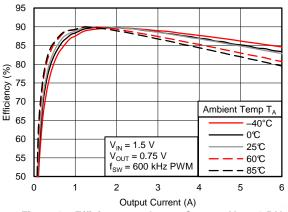
Figure 17. Efficiency vs. Output Current,  $V_{IN} = 1.5 \text{ V}$
