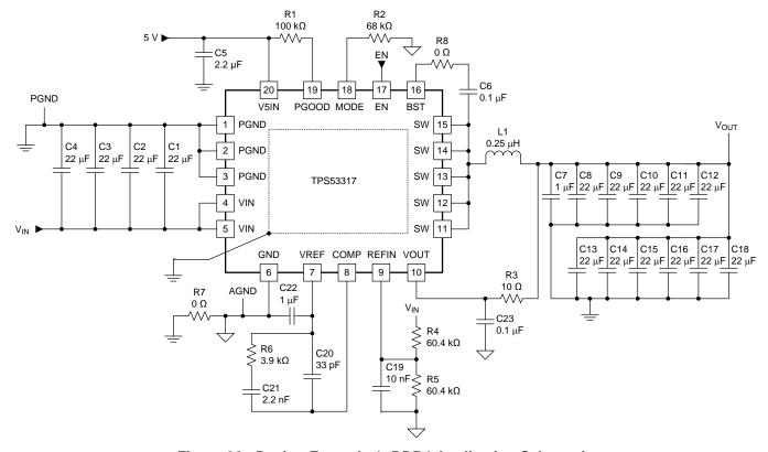
Figure 32. Design Example 1: DDR4 Application Schematic
