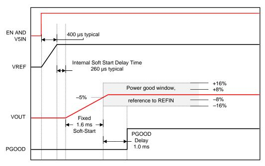
Figure 12. Non-Tracking Startup Timing
