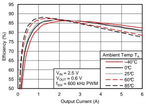
Figure 18. Efficiency vs. Output Current,  $V_{IN} = 2.5 \text{ V}$
