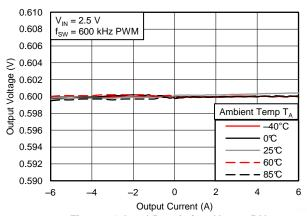
Figure 24. Load Regulation, V<sub>IN</sub> = 2.5 V
