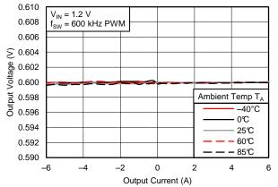
Figure 22. Load Regulation, V<sub>IN</sub> = 1.2 V
