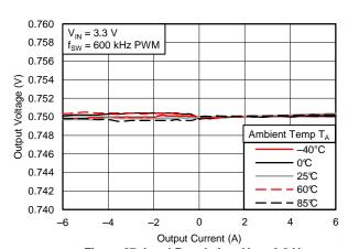
Figure 27. Load Regulation,  $V_{\rm IN}$  = 3.3 V
