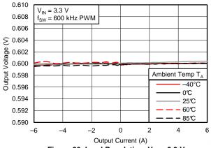
Figure 26. Load Regulation,  $V_{IN} = 3.3 \text{ V}$
