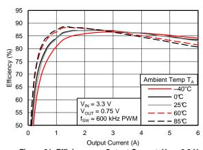
Figure 21. Efficiency vs. Output Current,  $V_{\text{IN}}$  = 3.3 V
