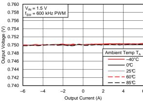
Figure 23. Load Regulation, V<sub>IN</sub> = 1.5 V
