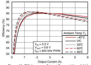
Figure 20. Efficiency vs. Output Current,  $V_{\text{IN}}$  = 3.3 V
