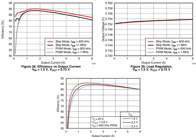
Figure 30. Efficiency vs. Output Current, V<sub>OUT</sub> = 0.9 V
