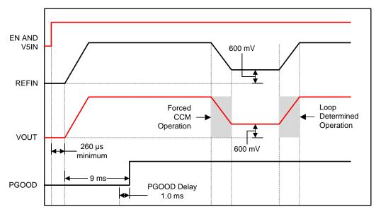
Figure 15. Tracking Startup Timing
