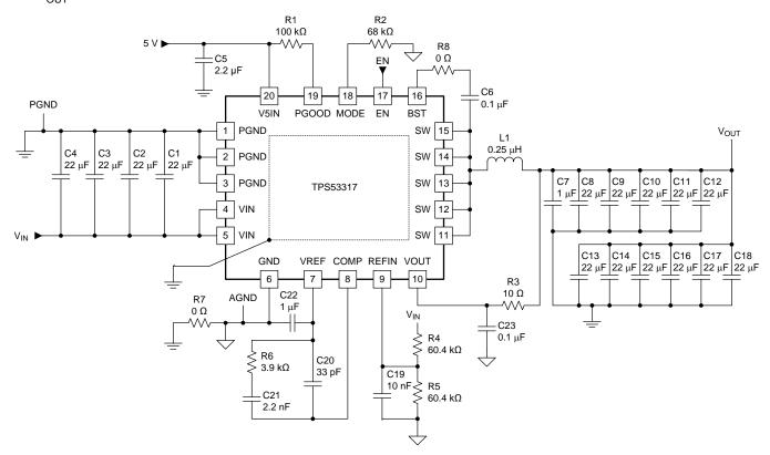
Figure 39. Design Example 2 Schematic: DDR3 Application
