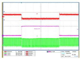
Figure 9. Load Regulation for 1.5-V Input, 0.75-V Output (Droop Configuration)
