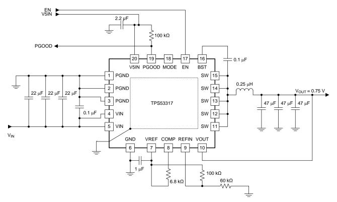
Figure 2. Application Using Droop Configuration
