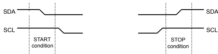
Figure 14-3. START and STOP Conditions
