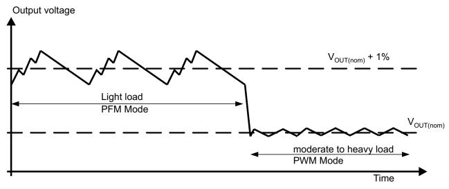
Figure 16. PFM Voltage Positioning
