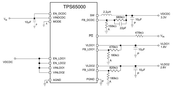
Figure 24. Typical TPS65000 Application Schematic
