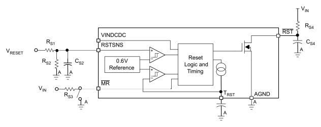
Figure 22. SVS Block Diagram
