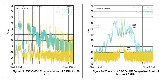
Figure 19 to Figure 20 shows the advantage of SSC with the frequency spectrum centering on the nominal frequency 2.25 MHz. The blue spectrum is the result of the spread change. The figures show the harmonic spectrum is attenuated 10 dB comparing to the same device without SSC.
