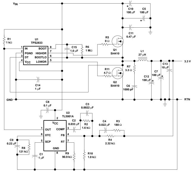
Figure 16. 3.3 V 3 A Synchronous-Buck Converter Circuit
