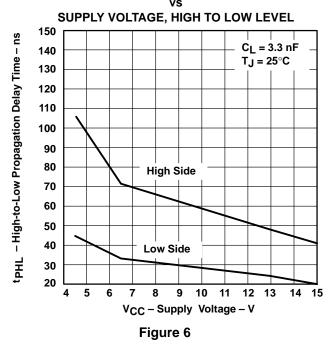
**HIGH-TO-LOW PROPAGATION DELAY TIME**
