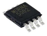
MORN series resistor networks feature four isolated resistors with standard 0.65 mm (25.6 mil) pitch lead spacing. The networks feature close TCR tracking and tight ratio tolerance and are ideally suited for unity gain operational amplifier circuitry. The standard resistance offerings listed are available for immediate delivery.
