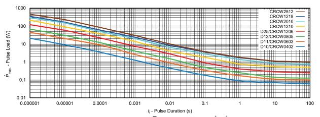
Maximum pulse load, single pulse; applicable if  $\overline{P} \to 0$  and n < 1000 and  $\hat{U} = \hat{U}_{max.}$ ; standard operation mode, for permissible resistance change equivalent to 8000 h operation
