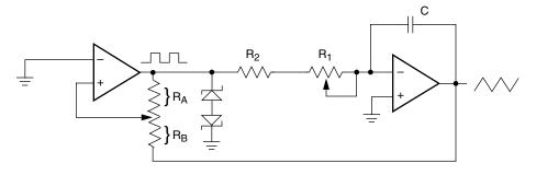
frequency  $\propto R_1, R_2, C$ amplitude  $\propto R_A, R_B$
