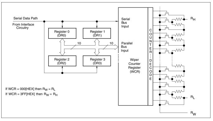
Figure 1. Detailed Potentiometer Block Diagram
