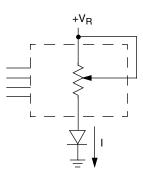
Two terminal Variable Resistor; Variable current
