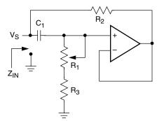
$$\begin{split} Z_{IN} = R_2 + s \; R_2 \; (R_1 + R_3) \; C_1 = R_2 + s \; \text{Leq} \\ (R_1 + R_3) >> R_2 \end{split}$$
