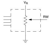
Three terminal Potentiometer; Variable voltage divider
