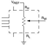
Three terminal potentiometer; variable voltage divider
