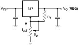
$V_{O}(REG) = 1.25V (1+R_2/R_1)+I_{adj}R_2$
