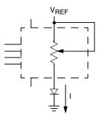
Two terminal variable resistor; variable current
