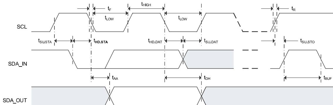
Figure 10. SCL: Serial Clock, SDA: Serial Data
