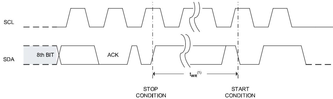
Notes: The write cycle time  $t_{WR}$  is the time from a valid stop condition of a write sequence to the end of the internal clear/write cycle.
