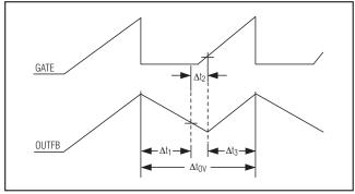
Figure 5. MAX6495/MAX6496/MAX6499 Timing
