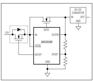
Figure 7. Overvoltage Limiter with Low-Voltage-Drop Reverse-Protection Circuit (MAX6496)
