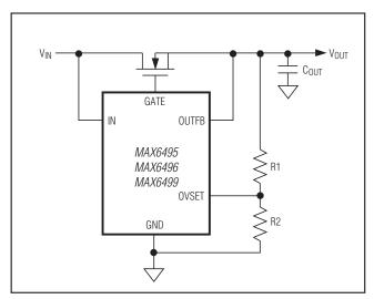
Figure 2. Overvoltage-Limiter Protection Switch Configuration
