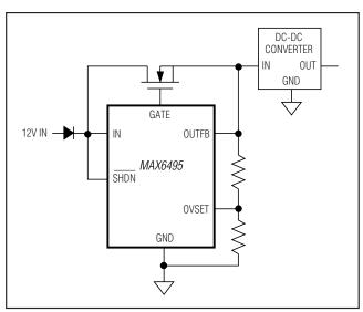
Figure 6. Overvoltage Limiter (MAX6495)
