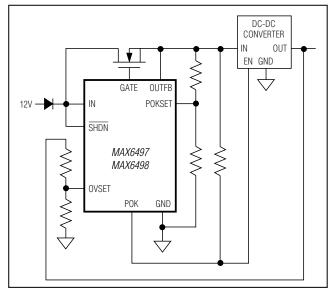
Figure 8. Overvoltage Protection to a DC-DC Converter (MAX6497/MAX6498)
