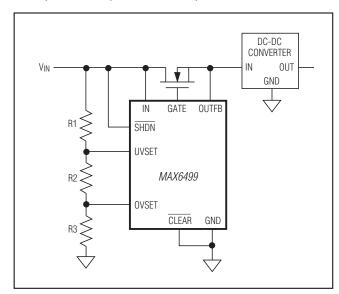
Figure 3. MAX6499 Window-Detector Circuit
