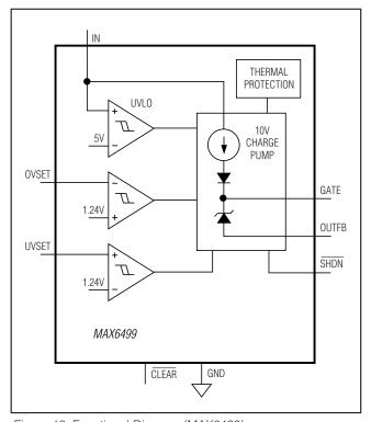
Figure 13. Functional Diagram (MAX6499)
