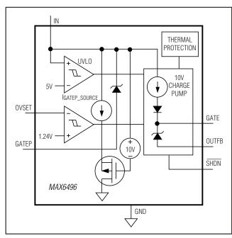
Figure 11. Functional Diagram (MAX6496)
