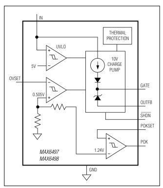
Figure 12. Functional Diagram (MAX6497/MAX6498)
