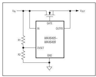
Figure 1. Overvoltage Threshold (MAX6495–MAX6499)
