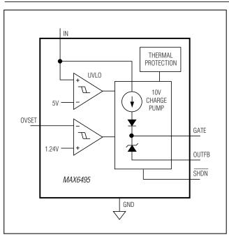
Figure 10. Functional Diagram (MAX6495)
