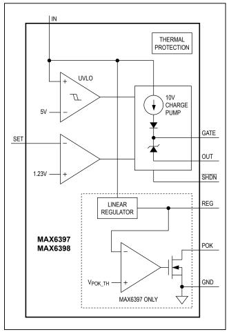
Figure 1. Functional Diagram
