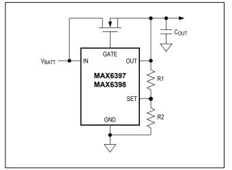
Figure 4. Overvoltage Limiter Protection Switch Configuration
