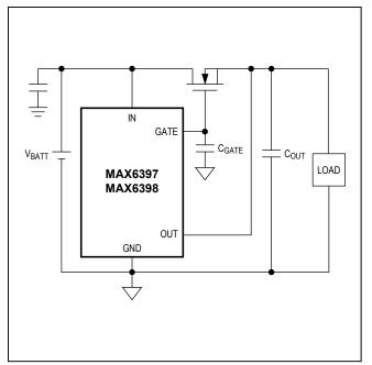
Figure 7. MAX6397/MAX6398 Controlling GATE Inrush Current
