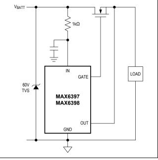
Figure 8. Protecting the MAX6397/MAX6398 Input from High-Voltage Transients
