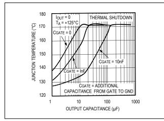
Figure 11. Junction Temperature vs. COUT
