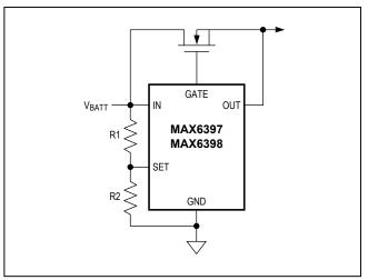
Figure 3. Overvoltage Switch Protection Configuration
