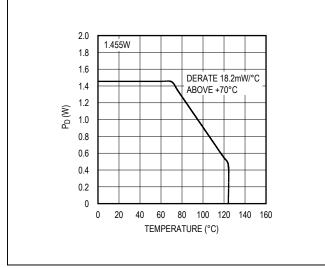
Figure 12. Maximum Power Dissipation vs. Temperature
