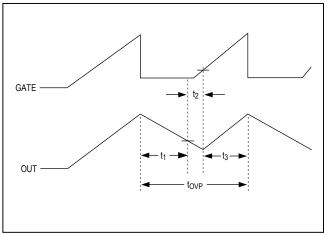
Figure 10. MAX6397/MAX6398 Timing Diagram
