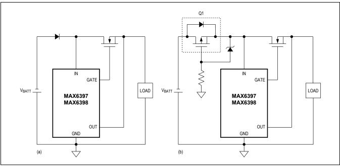
Figure 6. Reverse-Battery Protection Using a Diode or p-Channel MOSFET
