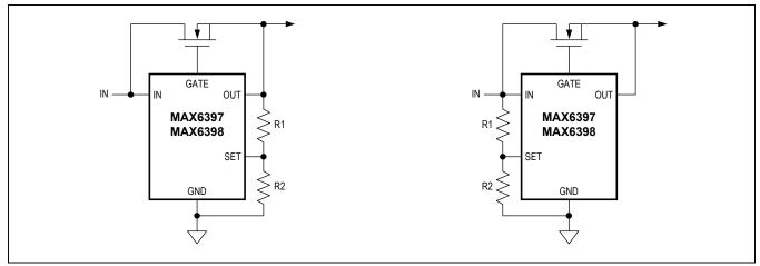
Figure 5. Setting the MAX6397/MAX6398 Overvoltage Threshold
