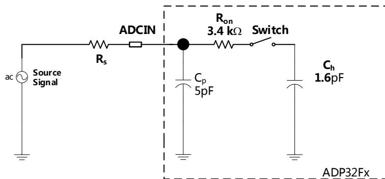
Typical Values of the Input Circuit Components:
