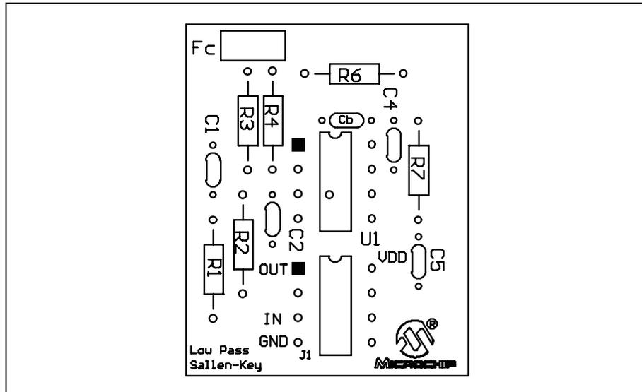
Figure 4.2: Filter Board Layout (Sallen-Key Configuration)
