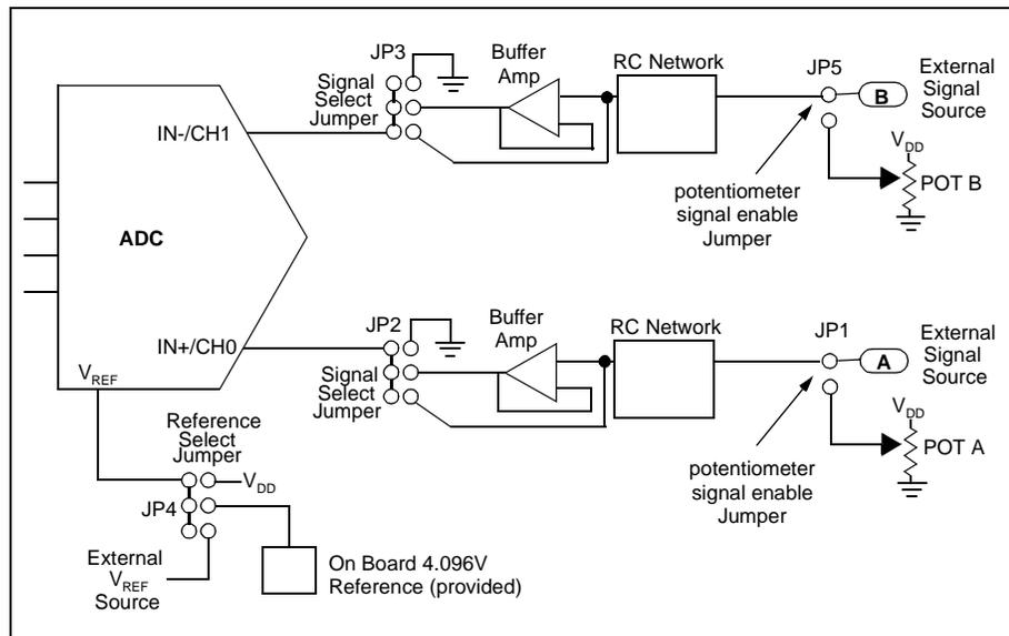
Figure 2.1: Basic Signal Chain for Single/Dual Daughter Board
