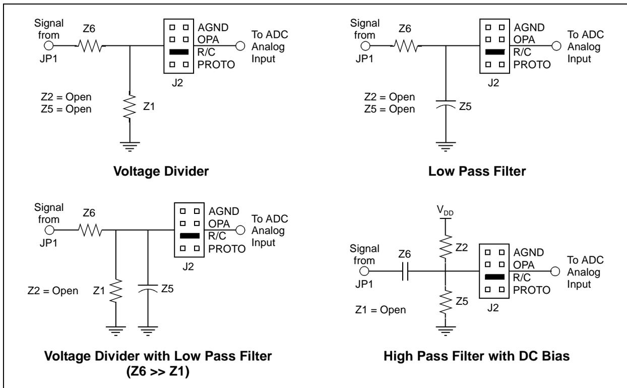
Figure 3.12: RC Network Circuit Examples using "A" Signal Path
