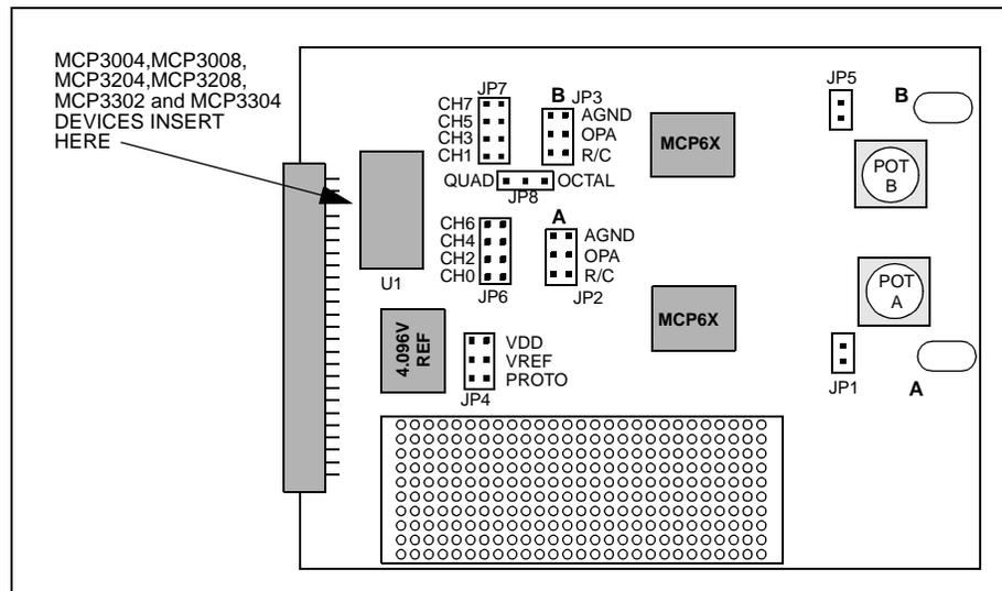
Figure 1.3: 14 and 16-pin ADC Board Device Locations for Quad/Octal Board
