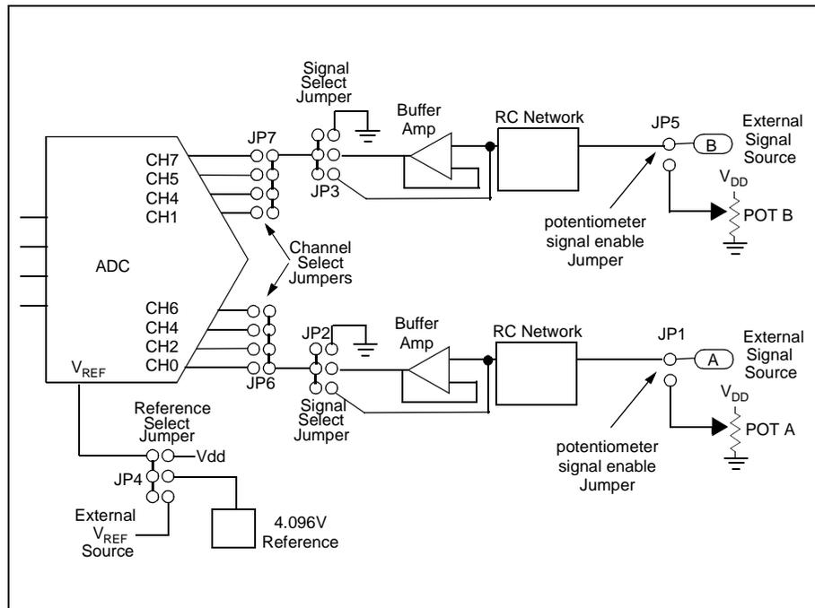
**Figure 3.1: Basic Signal Chain for Quad/Octal MCP3XXX Daughter Board**
