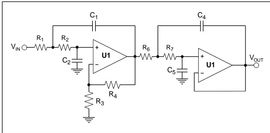
Figure 4.3: Filter Board Schematic
