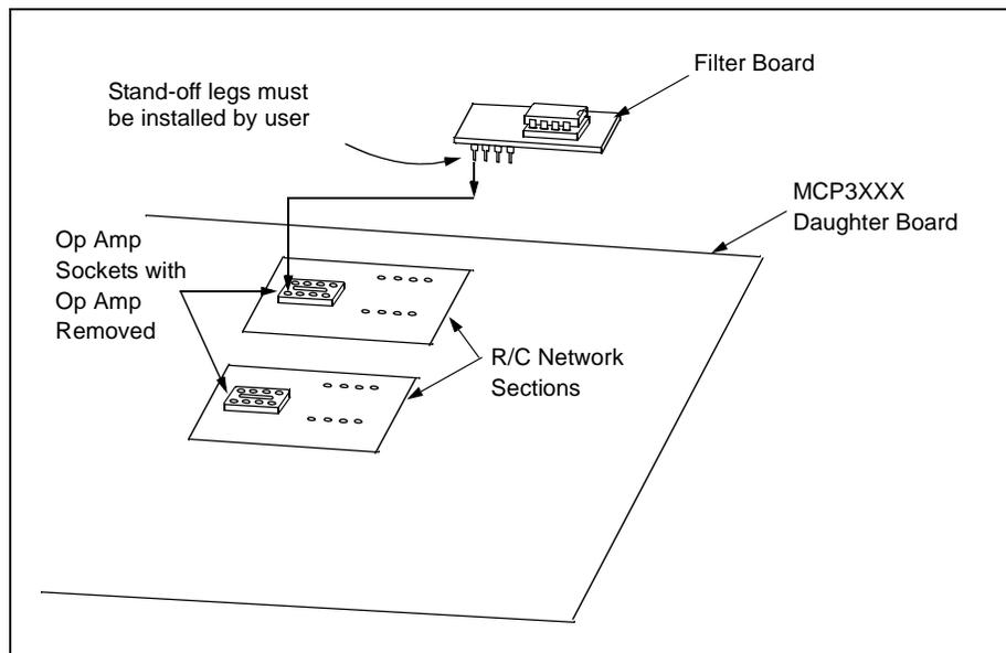
**Figure 4.1: Inserting Filter Board into Op Amp Socket**
