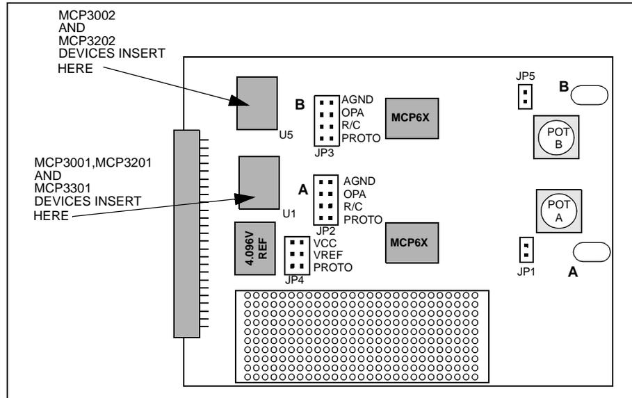
Figure 1.2: 8-lead ADC Board Device Locations for Single/Dual Board
