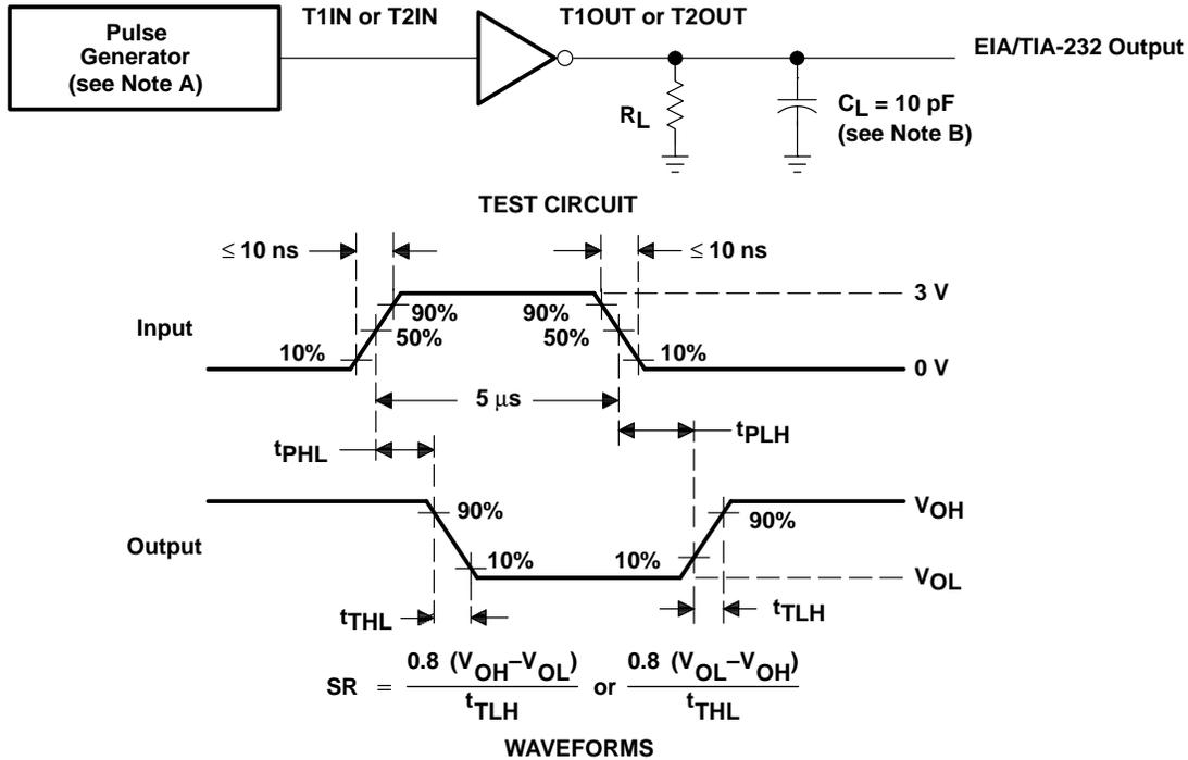
NOTES: A. The pulse generator has the following characteristics:  $Z_O = 50\text{ }\Omega$ , duty cycle  $\leq 50\%$ .
