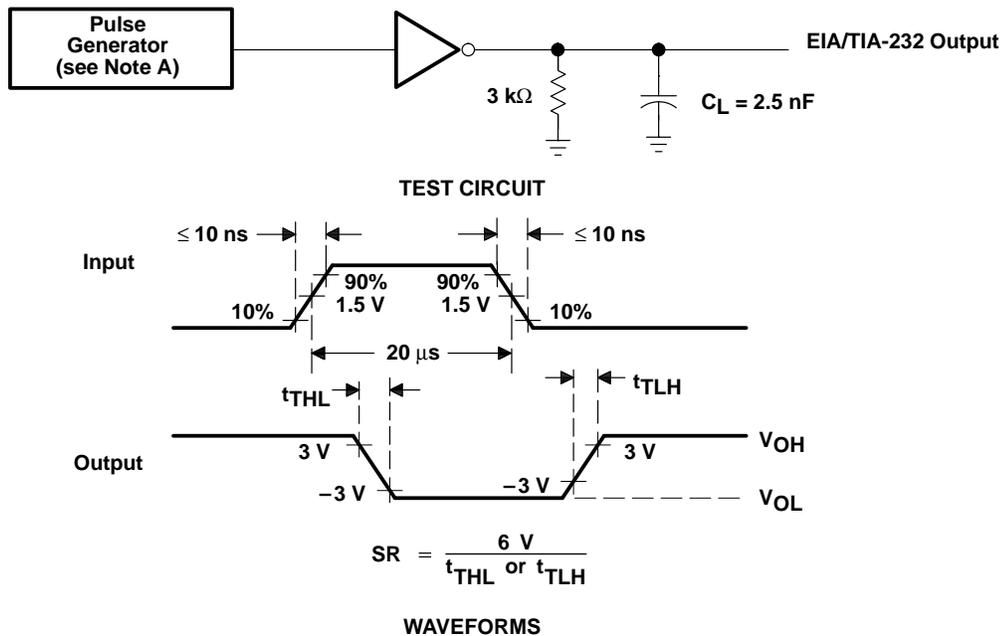
NOTE A: The pulse generator has the following characteristics:  $Z_O = 50\text{ }\Omega$ , duty cycle  $\leq 50\%$ .
