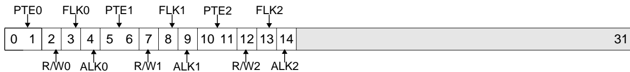
Figure 2-6. Bridge Error Status Register 0 (POB0_BESR0)
