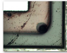
Corrosion failure after 168 hours Competitor 2
