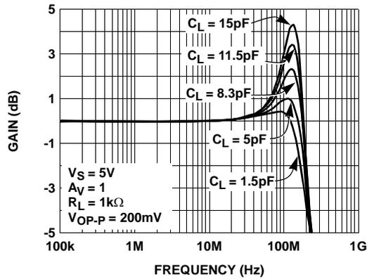
FIGURE 5. SMALL SIGNAL FREQUENCY RESPONSE FOR VARIOUS  $C_L$
