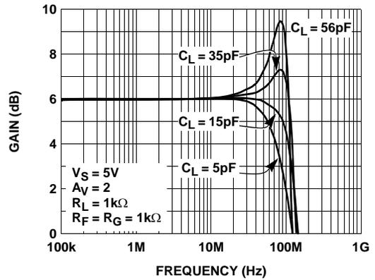
FIGURE 6. SMALL SIGNAL FREQUENCY RESPONSE FOR VARIOUS  $C_L$
