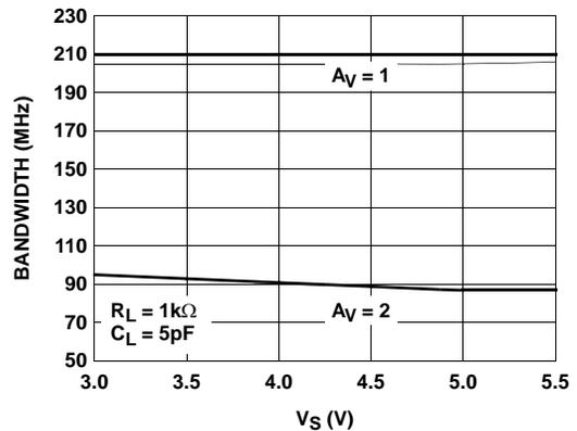
FIGURE 10. SMALL SIGNAL BANDWIDTH vs SUPPLY VOLTAGE
