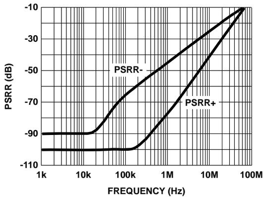
FIGURE 13. POWER SUPPLY REJECTION RATIO vs FREQUENCY
