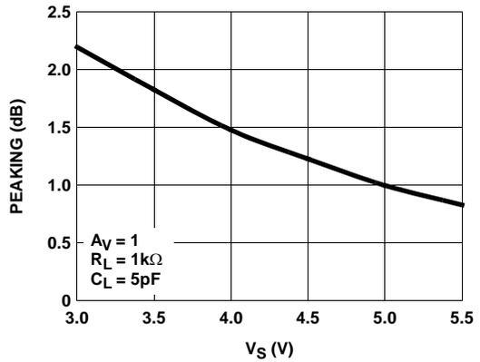
FIGURE 12. SMALL SIGNAL PEAKING vs SUPPLY VOLTAGE
