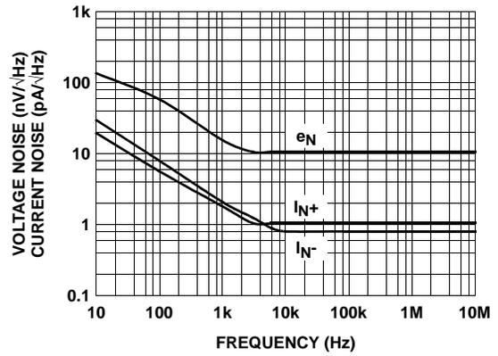
FIGURE 18. VOLTAGE AND CURRENT NOISE vs FREQUENCY
