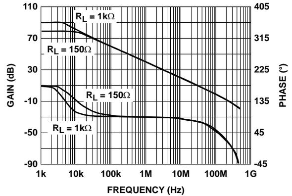
FIGURE 8. OPEN LOOP GAIN AND PHASE vs FREQUENCY
