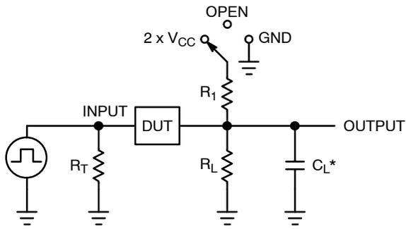
$C_L$  includes probe and jig capacitance
