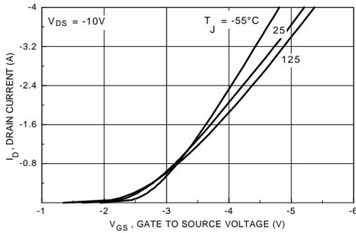
Figure 5. Transfer Characteristics.
