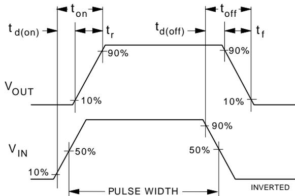
Figure 12. Switching Waveforms.
