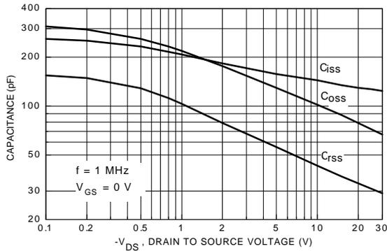
Figure 9. Capacitance Characteristics.
