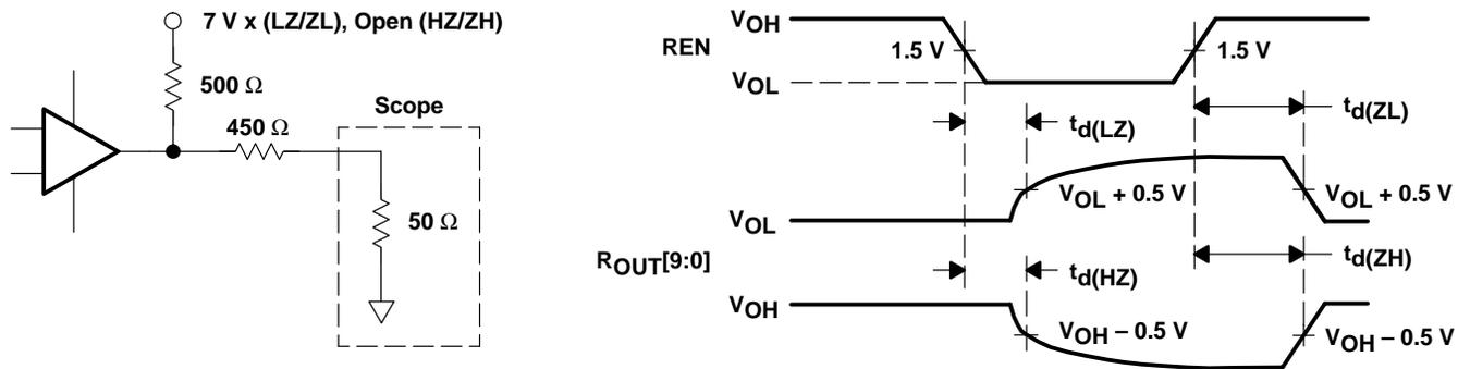
Figure 14. Deserializer High-Impedance-State Test Circuit and Timing
