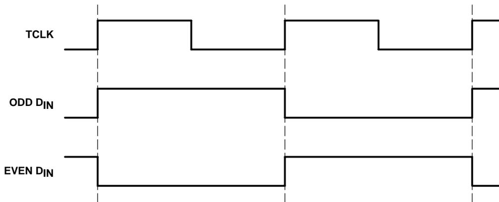
**Figure 2. Worst-Case Serializer I<sub>CC</sub> Test Pattern**
