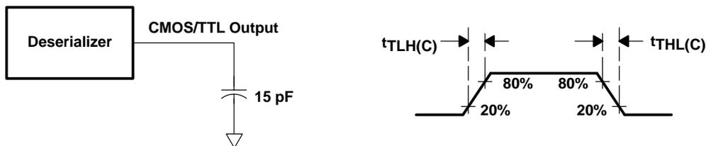
Figure 5. Deserializer CMOS/TTL Output Load and Transition Times
