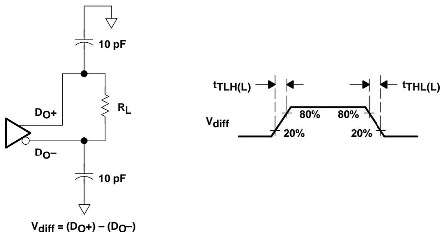
Figure 4. Serializer LVDS Output Load and Transition Times
