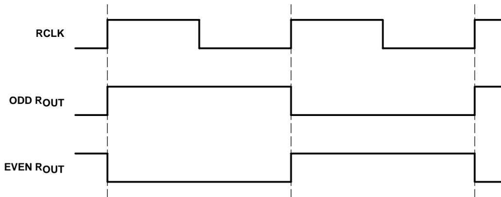
**Figure 3. Worst-Case Deserializer I<sub>CC</sub> Test Pattern**
