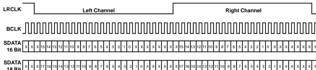
**Figure 2–1. Philips I<sup>2</sup>S Protocol Serial PCM Data Format**
