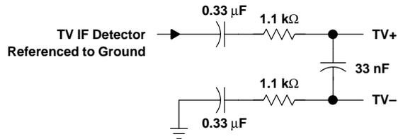
Figure 4–1. De-Emphasis 75  $\mu$ s Low-Pass Filter at 2.12 kHz
