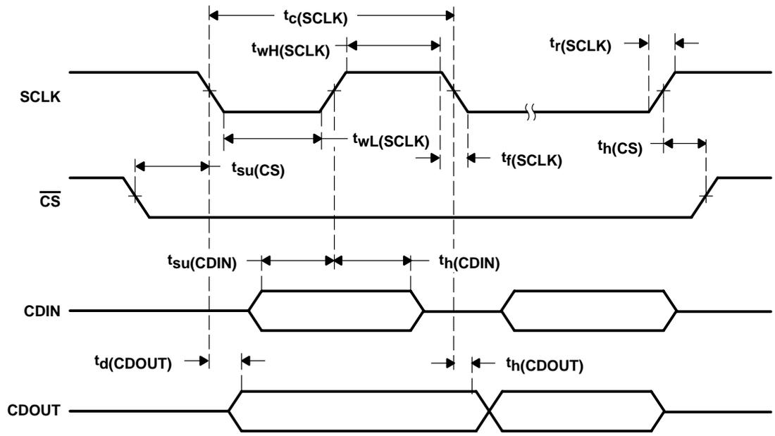
Figure 3-2. SPI Serial Control Port Timing
