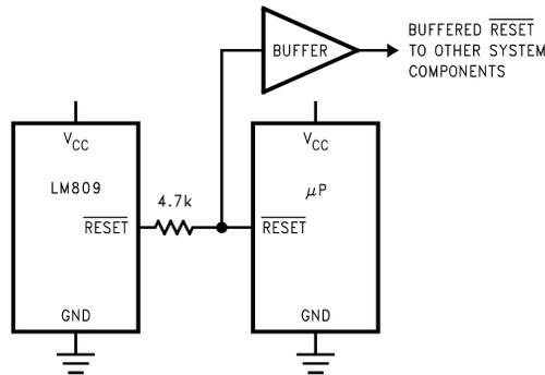
Figure 11. Interfacing to Microprocessors with Bidirectional Reset I/O
