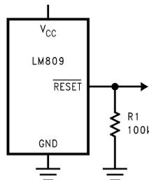
**Figure 9.  $\overline{\text{RESET}}$  Valid to  $V_{CC} = \text{Ground}$  Circuit**
