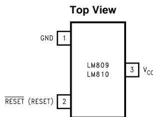
**Figure 1. 3-Lead SOT-23-3 Package**
